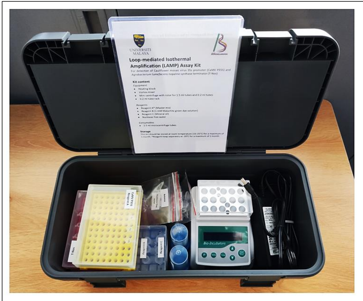
Rajah 4.9. Susunan kit ujian loop-mediated isothermal amplification (LAMP) .
